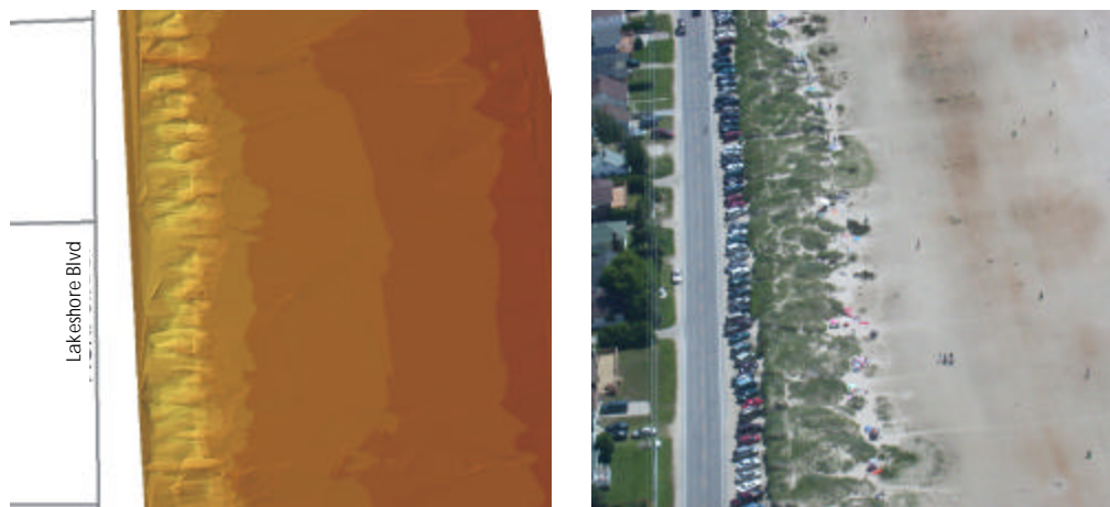
Example of 3 dimensional image of the dunes at Sauble Beach showing the physical structure of the dunes. This research, conducted by researchers from the Department of Geography at Wilfred Laurier University, will help in our understanding of erosion and accretion dynamics at Sauble Beach. (3-D Image provided by C. Houston).
